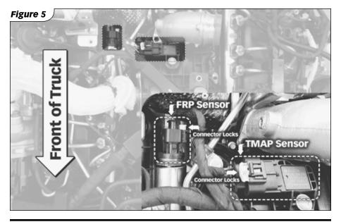
**7.** For each connector, slide the yellow connector lock away from the sensor body, then depress the connector latch and slide the connector off the sensor.
