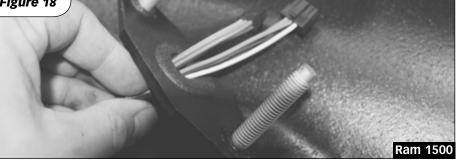
**19.** Re-install the block off plate mounting nuts onto the studs from the inside of the cab. Then carefully pull the remaining free length of the Derringer Starter Cable through the firewall. Be sure to leave a little slack on the engine bay side of the firewall.
