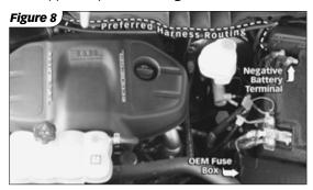
**12.** Connect the Derringer module to the sensor harness.
