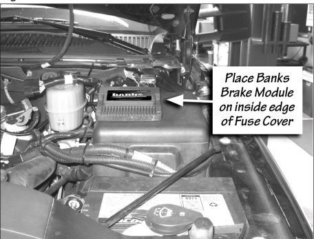
Figure 12 Placement of Banks Tuner on top of the Fuse Box.
