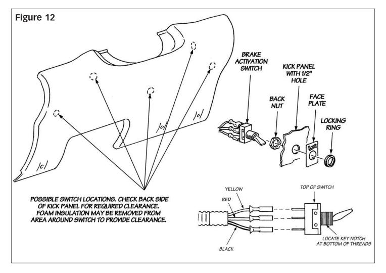
Note: Be sure to cut the correct color wire. There may be a white wire with a red tracer in close proximity to the cruise control wire and may easily be mistaken for the right lead. Crimp the male and female 1/4" spade connectors to each end of the cut wires. Connect the two brown wires from the harness to feed spade connector.
