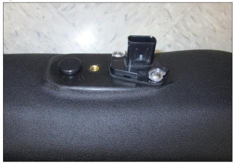
(41872) using the two provided 6-32 screws (91719). Install the Map Sensor Plug (41876) into the adjacent sensor port.
