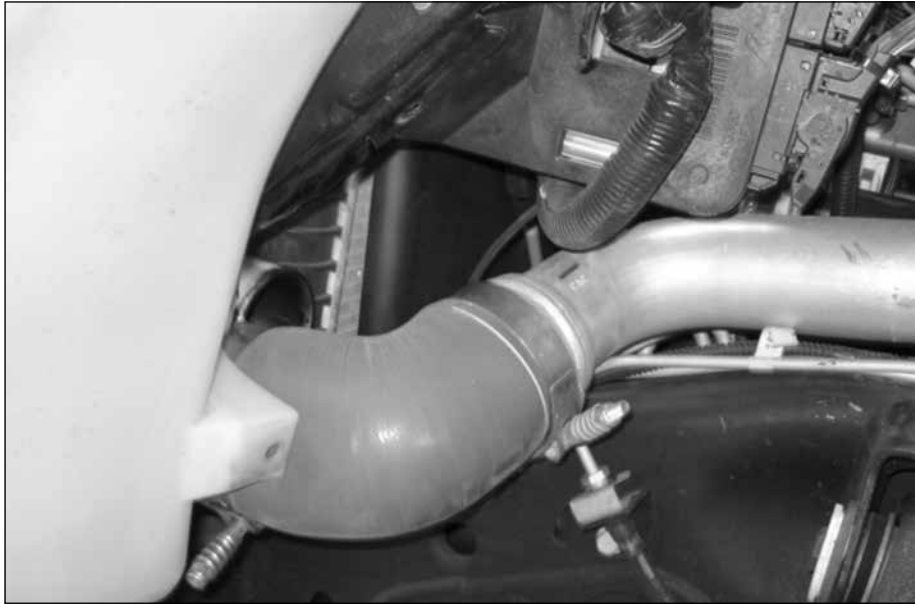
Figure 17 Drivers side boost hose
