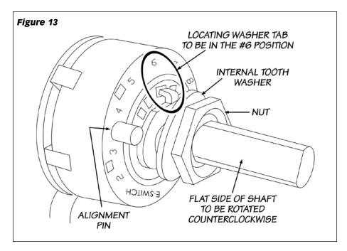
washer and nut. Snug the washer; be careful not to over torque the nut and damage the plastic threads.
