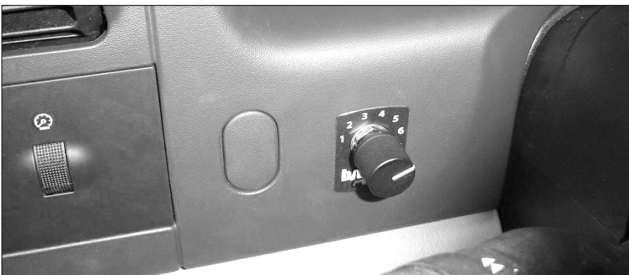
Figure 50: Finished installation of the Power Level Selector Switch on 2005-07 model year vehicles
