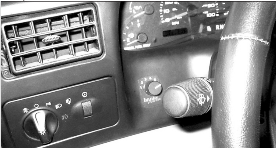
Figure 50: Finished installation of the Power Level Selector Switch on 2005-07 model year vehicles
