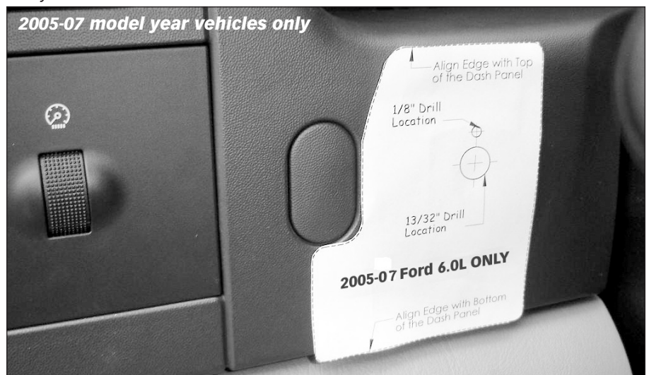
Figure 47 Template taped to front of dash on 2005-07 model year vehicle, ready to be drilled.
