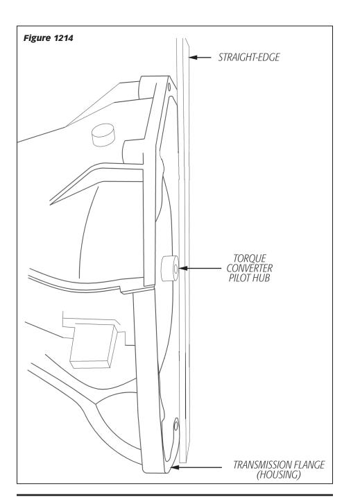
properly and engage the transmission input shaft splines, then carefully work the torque converter onto the transmission input shaft until it is recessed behind the front transmission mounting flange.
