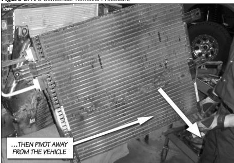
Figure 5. A/C Condenser Removal Procedure
