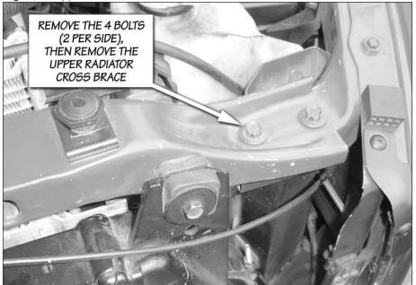
Figure 3. Relocation of the Upper Driver Side A/C Condenser Mounting Bracket
