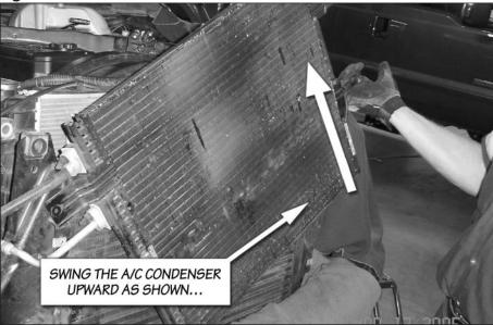
Figure 4. A/C Condenser Removal Procedure
