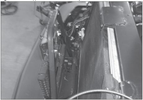
Figure 7: Upper Charge Air Cooler (CAC) attachment bolt
