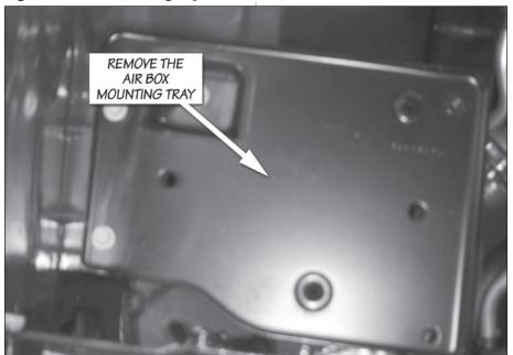
Figure 9: Air box support bracket
