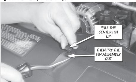
Figure 1: Removal of push-in retaining pins
