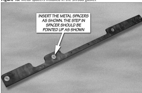
**Figure 15:** Metal spacers installed in the shroud gasket
