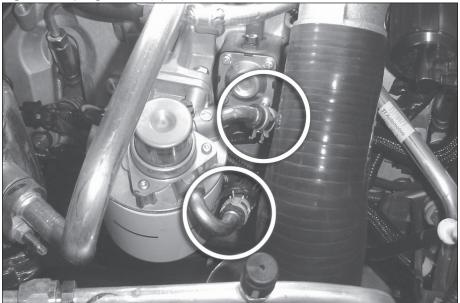
**49.** Install the driver and passenger side boost tubes. New clamps are provided for the intake manifold hose to boost tube connection and the turbo hose to boost tube connection. All other locations reuse the factory clamps. Tighten the clamps to 75 in-lbs. The following hoses are used at each location:
