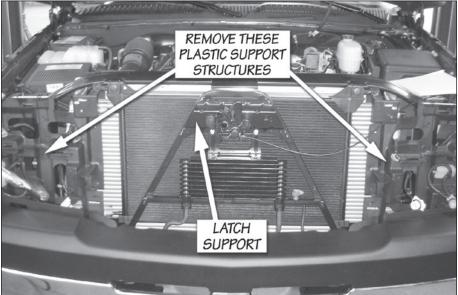
**Figure 4:** Removal of headlamp/parking lamp assembly support structures
