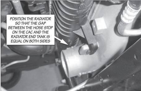
Figure 13: Gap between the CAC hose stop and radiator end tank
