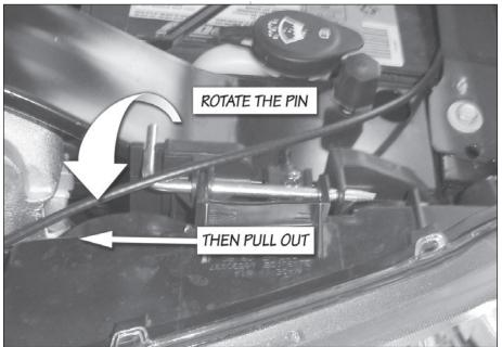
Figure 3: Parking lamp assembly removal
