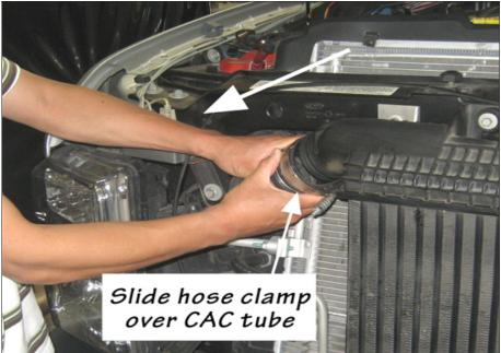
Figure 3 Disconnecting the Driver Side CAC Tube
