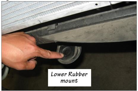
Figure 9 Connecting Fuel Cooler Radiator to Banks Techni-Cooler
