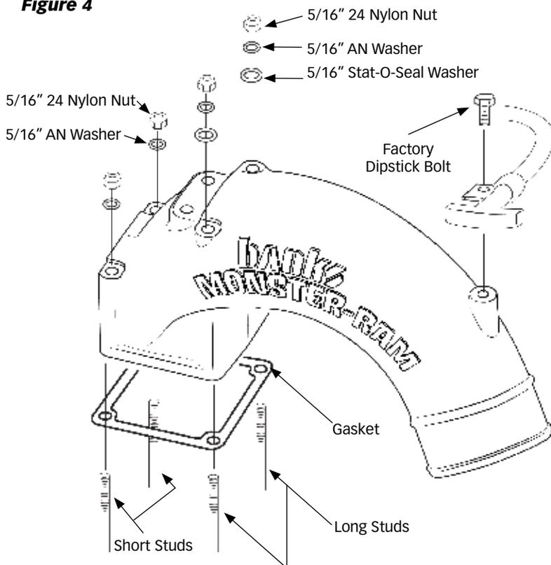
**14.** Slide the second provided intake gasket over the four studs and set the Monster-Ram in place on the studs. Twist a Stat-o-seal washer over the two driverside studs, then over each stud install a flat  $\frac{5}{16}$ " AN washer. Install a  $\frac{5}{16}$ " - 24 nylock nut on each stud and tighten all four evenly between 11-12.5 ft-lb (140 to 150 Inch Pounds) See **Figure 4**.
