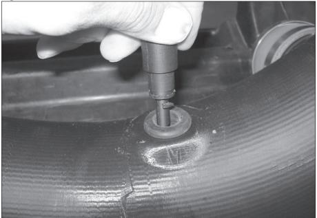
**14.** Locate the supplied rubber AIT grommet and install in the air intake tube. Install the AIT sensor flush into the grommet on the air intake tube. See **Figure 6**.
