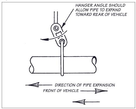
Muffler outlet. Lightly tighten the rear muffler hanger clamp to secure the front tailpipe. Install the Exhaust clamp onto the front tailpipe outlet. Install the rear tailpipe inlet into the front tailpipe outlet. Start the rear tailpipe hanger pin into the corresponding vehicle rubber hanger. Lightly tighten the exhaust clamp to secure the rear tailpipe.
