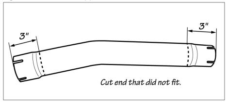
**7.** Locate the supplied Banks Intermediate pipe. Both ends of Banks intermediate pipe are size differently for different model applications. Fit Banks intermediate pipe over the Factory cut intermediate pipe. If one end does not fit over the Factory pipe try the other end. Insure that Banks intermediate pipe fits over the Factory pipe.
