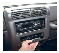
**5.** Remove coin tray from center console bezel by carefully grinding five plastic welds. Take care while grinding as to not damage the center console bezel.
