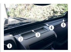
**2.** Remove ashtray by pressing on tab to release and pulling forward.
