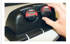
**7.** Place dash pod with gauges and/ or accessories on top of dash with leading edge on top of A/C vents. Secure dash pod to dash with two screws from step #3 in holes on back edge of dash pod.
