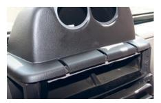
**8.** Reinstall center console bezel with the top edge over dash pod by aligning clips and pressing firmly until secured. Reinstall screw behind ashtray.
