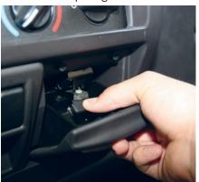
**3.** Use a #2 Phillips head screwdriver to remove two screws behind coin tray and one screw behind ashtray.
