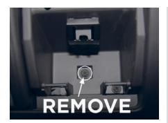
**4.** Remove center console bezel by carefully pulling forward on both top corners to release clips. Pull from center of bezel to remove.
