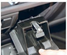
**10.** Reinstall trim with vent on top of dash under windshield by sliding back edge in place. Align clips and press firmly until secured.
