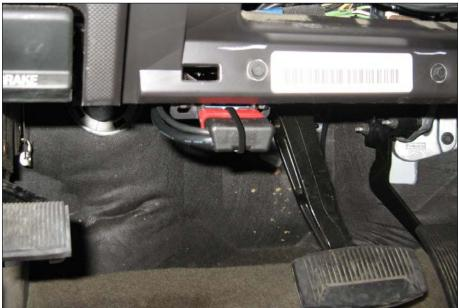
Figure 12 Brake Position Sensor location under dash
