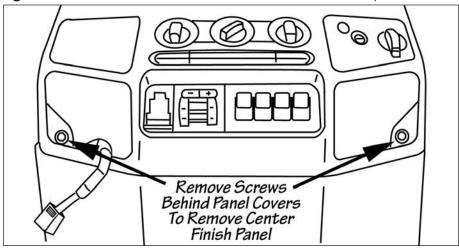
Figure 17 Removal of the Instrument Cluster Panel
