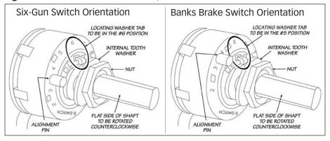
Figure 21 Finished installation of the Six-Gun/Banks Brake Switch
