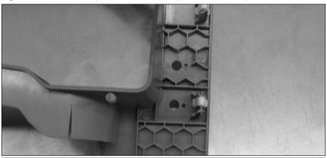
**15.** Route the Six-Gun switch's cable to the wire harness that was routed into the passenger compartment from the Six-Gun Diesel Tuner, and plug the 2-pin connector into the corresponding connector on the Six-Gun harness.
