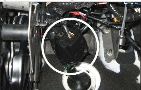
Figure 15 Banks Brake Module mounting location
