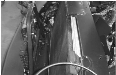
Figure 2.8 Upper Intercooler (CAC) Attachment Bolt.
