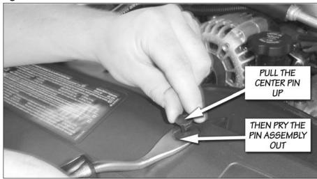
Figure 2.3 2006-07 LBZ: Headlamp Assembly Removal
