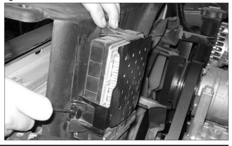
Figure 2.7 Latch Support Moved Out of the Way
