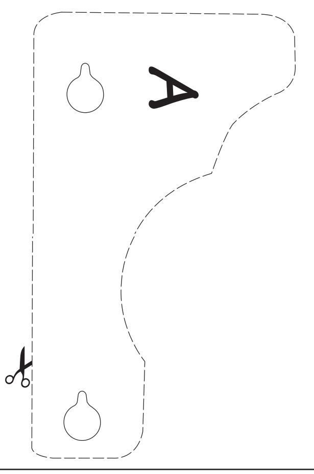
**Fig 2.13.** Trim template for the air box-mounting bracket.
