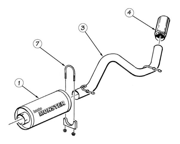
Figure 1.1 General Assembly Banks Split-Dual Monster Exhaust, Split-Dual
