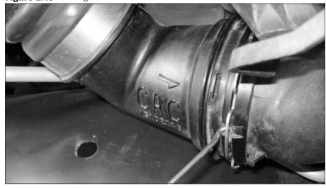
Figure 2.16 Passanger side boost tube
