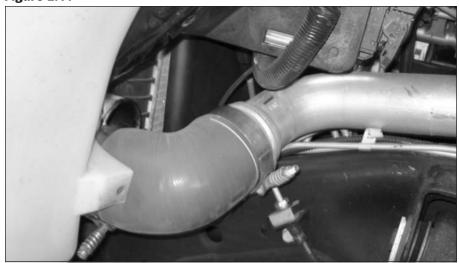
Figure 2.15 Passanger side boost tube
