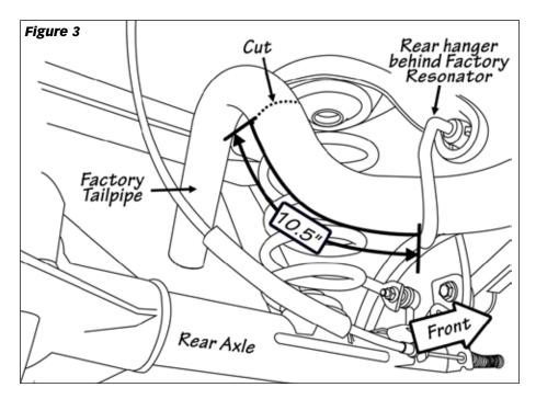
NOTE: Begin cutting just where the tubing begins to bend at the top. Try to leave as much straight tailpipe to receive Banks Front tailpipe.
