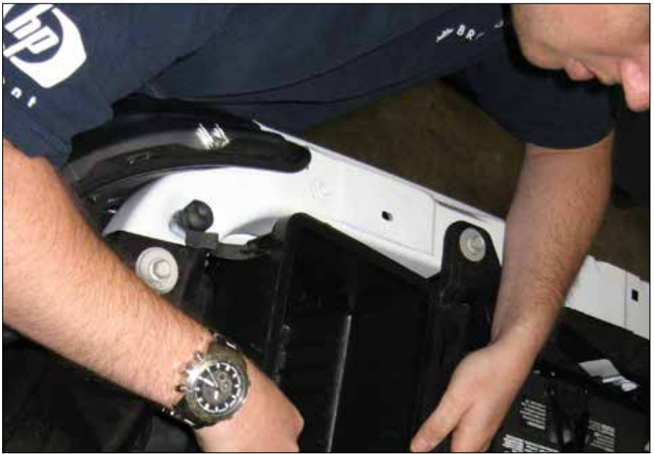
Figure 7- Removal of the stock air filter housing
