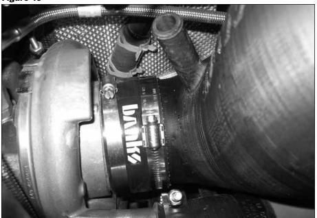
NOTE: The compressor supply and return lines may need to be slightly bent away from Banks air housing to provide clearance. Be careful not to break the condenser lines when adjusting clearance. See **Figure 11**.
