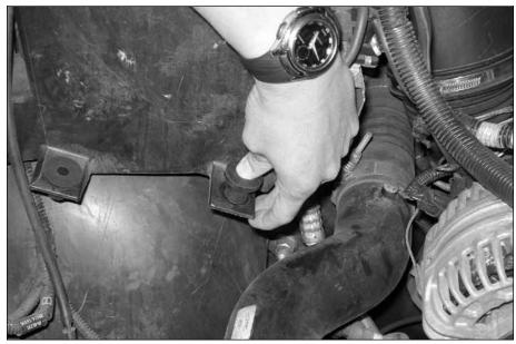
**7.** Install the supplied rubber Well-Nut as shown in **Figure 5**. Install flange side up, flush with bracket.
