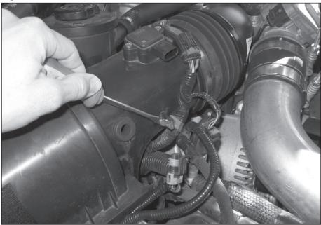
**9.** Push the air cleaner bellows away from the air filter housing while pulling up on the MAF side of the air filter. Lift and remove the air filter housing in the direction shown in **Figure 7**.
