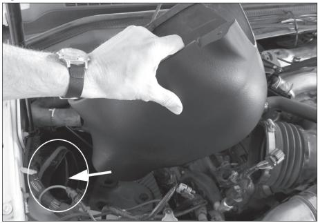
rubber isolators in the support bracket. Make sure to push the Filter Housing all the way down into the rubber isolators.
