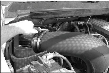
Figure 7- Installed Banks Ram-Air Intake System
