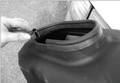
**8.** Install Banks filter hose clamp (Item 8) onto the Banks filter cuff (Item 2). Place Banks Filter into Banks filter housing.
