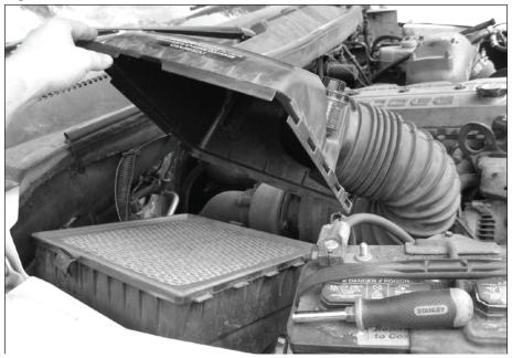
Figure 4- Removal of filter housing bottom
