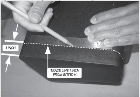
Figure 7-For Banks Super Scoop Installation Only
