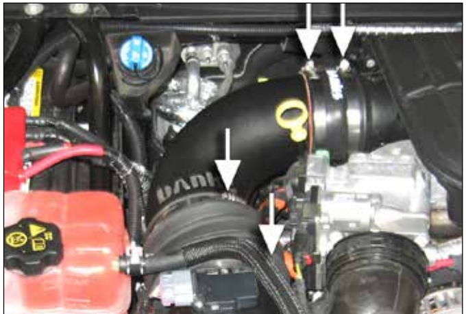
Figure 8- Secure Banks Intake Tube
