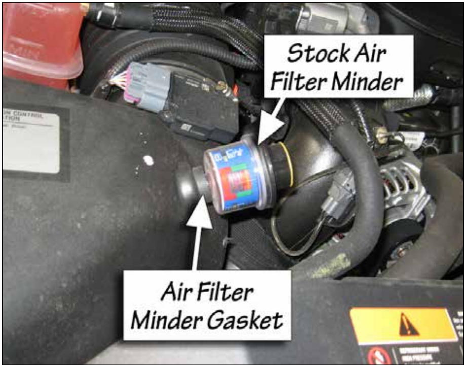
Figure 6- Remove Stock Air Filter Minder & Air Filter Minder Gasket
