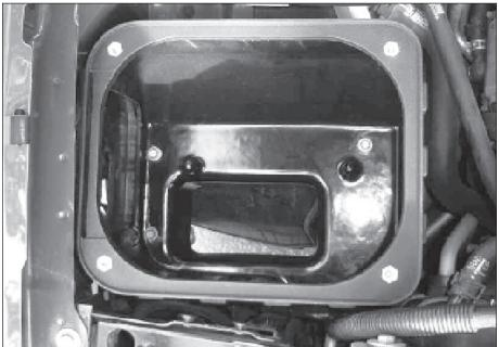
Figure 4-Install Banks MAF Gasket
