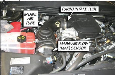
Figure 1- Seperate Intake Air Tube from Stock Air Box Cover
