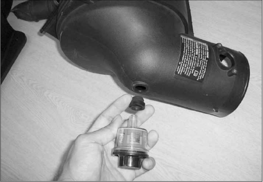
Figure 5- Remove Stock Air Filter Minder & Air Filter Minder Gasket
