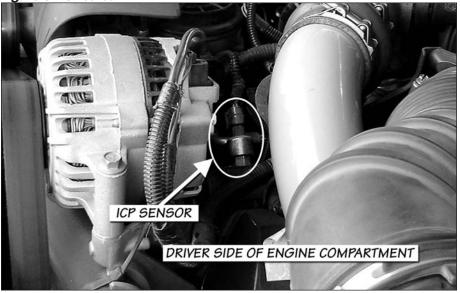
Six-Gun ICP wiring harness. Doublecheck that both connectors are properly indexed and latched securely.
