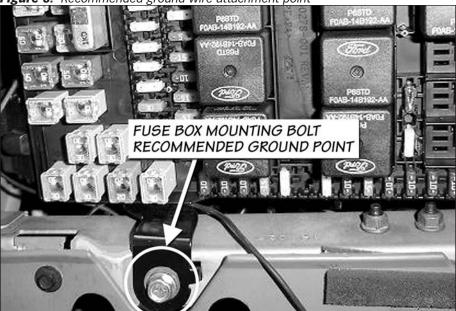
in the previous step. Route the red (RED) wire out through the bottom of the fuse box and reinstall the fuse box cover. (It may be necessary to bend the fuse tap/connector and route the wire around several fuse box components to allow clearance for the fuse box cover to snap back into place.)
