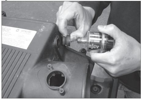
removed air filter minder and install into the rubber grommet. Make sure air filter minder is installed flush to rubber grommet. See **Figure 14**.
