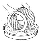
NOTICE: NEVER use gasoline, steam, caustic solutions, strong detergents, high-pressure nozzles, or cleaning solvents to clean the filter element. All of these can cause harm to the filter media as well as SHRINK and HARDEN the rubber end caps.
