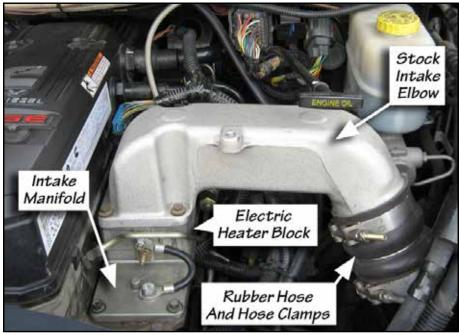
**7.** Remove the driver side boost tube, hoses and hose clamps. Retain the factory hose and hose clamps at the inlet of the factory driver side boost tube for reuse with Banks Boost Tube. The boost tube is the charge air ducting that routes air from the Charge Air Cooler (CAC) to the intake manifold.
