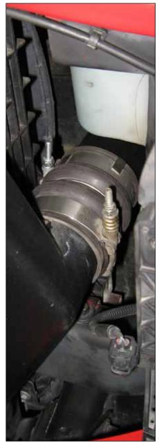
**10.** Make sure that the M8 ends go into the engine intake manifold. The two shorter studs go on the passenger side (closest to the valve cover). Apply the supplied thread lock compound at the M8 ends and hand-tighten the studs into the intake manifold.
