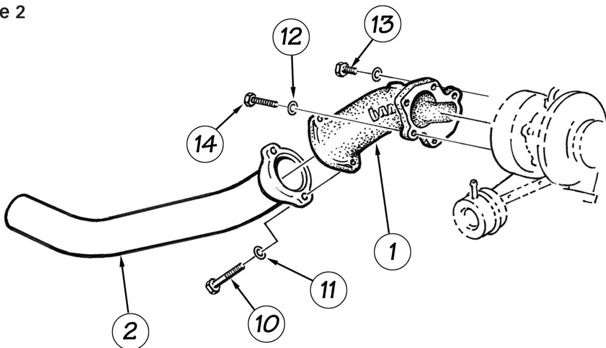
**12.** A. If the Banks Power Elbow was installed, Torque the two (2)  $\frac{7}{16}$ " turbine outlet pipe attach bolts to 15 ft-lbs. *NOTE: Do not use an impact wrench on these fasteners. The wide span of the two-bolt spherical flange creates sufficient clamping force when 15 ft-lbs is used. Exceeding this torque specification will not increase the sealing performance.*
