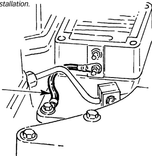
**9.** Install Banks driver side boost tube. The driver side tubes use a 3.5 inch diameter hump hose and Spring loaded clamps at the connection to the Banks Monster-Ram and re-use the factory hose and clamps at the CAC. Keep the hose clamps loose until the Monster Ram is installed. Cover the opening of the boost tube to prevent foreign objects from entering the boost tube during the installation.
