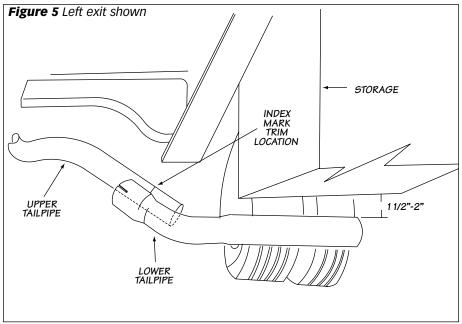
**13.** With the exhaust postioned properly, begin to tighten the clamps starting with the ones closest to the front of the vehicle and working your way back. Torque the 3/8" hardware and exhaust clamps evenly to 35 ft-lbs. Make sure that each slip is fully inserted (+/- 1/4"). All hanger pins should be facing forward (see **Figure 6**). Remove the protective covering from the tailpipe tip.
