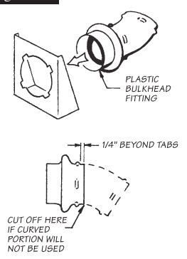
Drill four  $\frac{3}{16}$ " diameter holes through the air inlet hood bracket around the perimeter of the center hole. See Figure 5. If the bracket cannot be drilled while in place, it may be unbolted for drilling.
