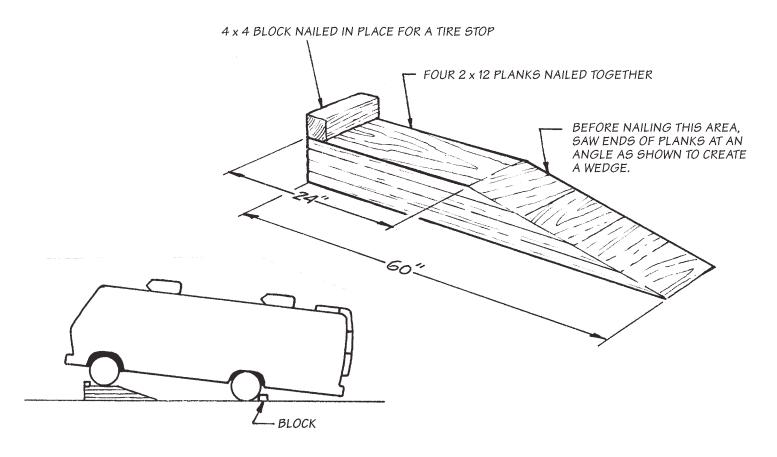
12. Raise front of vehicle on hoist or ramps. Note: Figure 9 shows how ramps may be constructed for this purpose.
