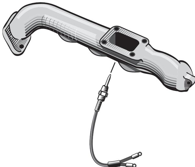
Mark a position on the exhaust manifold to locate the pyrometer sensor. Stuff a small shop towel or rag four to five inches into the exhaust manifold through the turbo mounting flange to prevent chips from entering the manifold while drilling and tapping.
