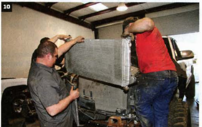
9&10. Then the intercooler can be removed, but it may take an extra set of hands. You may need a friend or two to lend a helping hand.
