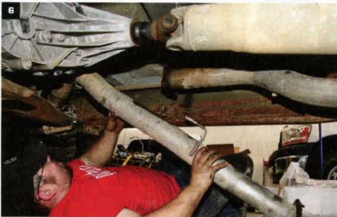
6 Zach Bruner removes the front section of the original 3.5-inch exhaust after removing the V-band clamp at the downpipe and mounting nuts at the four-bolt exhaust flange.
