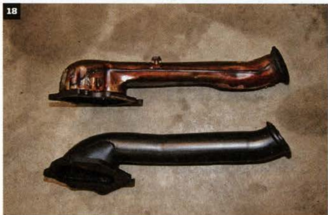
A side-by-side comparison of the original downpipe and the Pro Fab Performance downpipe shows the serious restriction that is eliminated with the new fabricated downpipe.
