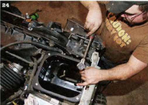
24 Bruner mounts the filter housing to the airbox support bracket after removing the airbox mounting tray. The air filter is now able to draw in outside air from the underside of the fender well.
