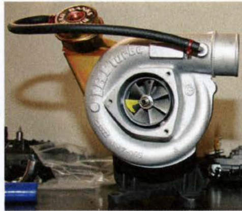
Fleece Performance Engineering's LB7 turbo may look stock, but it's not. It boasts a 63mm billet compressor wheel and high-flow inconel turbine wheel that can deliver up to 600 hp.
