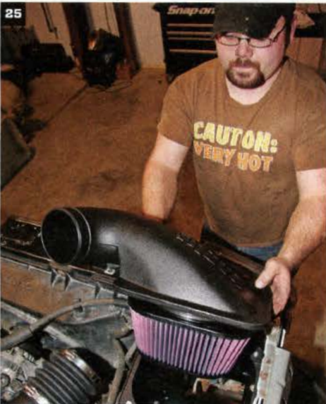
25 The large, reusable filter is mounted directly to the lid, with its integrated air inlet, to feed the engine plenty of filtered air.
