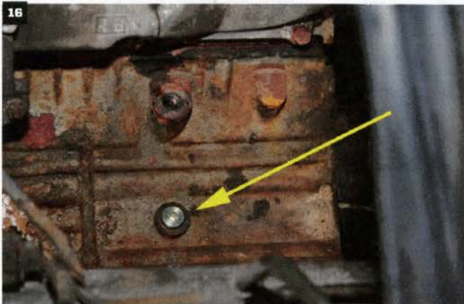
Don't forget to install the oil feed plug (see arrow) before you put the turbo back in—or you could have a real mess on your hands and also add a lot of extra work and time to your installation. Fleece supplies a new feedline that is fed from the oil galley on the front passenger's side of the engine block to be sure the turbo has plenty of lubrication.
