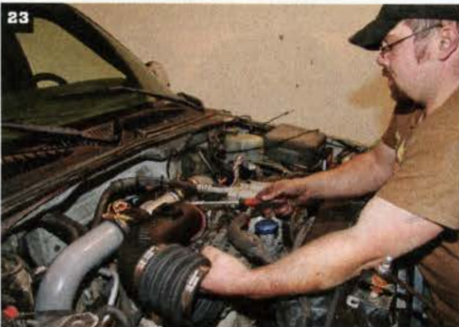
23 The Ram-Air intake features a smooth transition to the turbo inlet. Be sure to use the supplied O-ring, in addition to the factory O-ring, when installing the MAF sensor.
