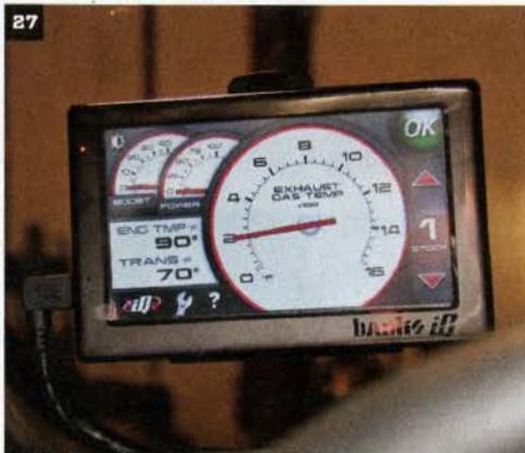
27 With the iQ's selectable gauge functionality, we can monitor several of the Duramax's vital signs while on the road, as well as all the additional functions and features built into the iQ.
