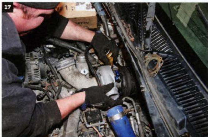
Hale drops the new turbo into position and bolts up the oil drain and turbo mounts before installing the up pipes. Be sure to use anti-seize compound on the nuts and bolts to make it easier to remove them in the future, if necessary.
