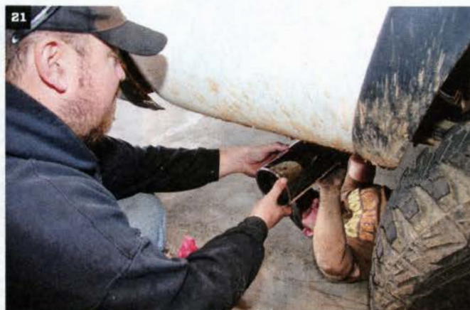
Newton and Bruner set the tailpipe angle and then install the 5-inch-diameter, polished stainless steel tip. We opted for the single side exit exhaust system, since it would be easiest to modify to clear the custom long-travel rear suspension we plan to install in the near future.
