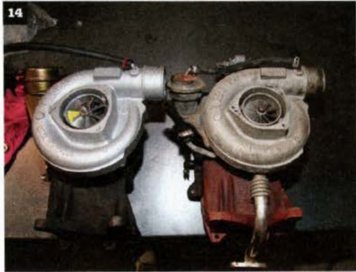
With the two turbos side by side on the workbench, it is easy to see the larger and more aggressive compressor wheel on the Fleece Performance Engineering 63mm LB7 Cheetah turbo. The Banks BigHead wastegate actuator is already installed on the new turbo to
