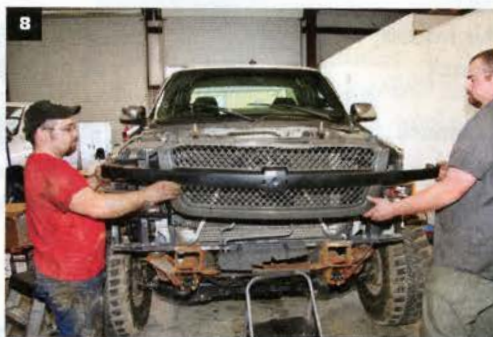
8 Before the old intercooler can be removed, the grille, lights, mounts and upper part of the core support need to be removed from the truck.
