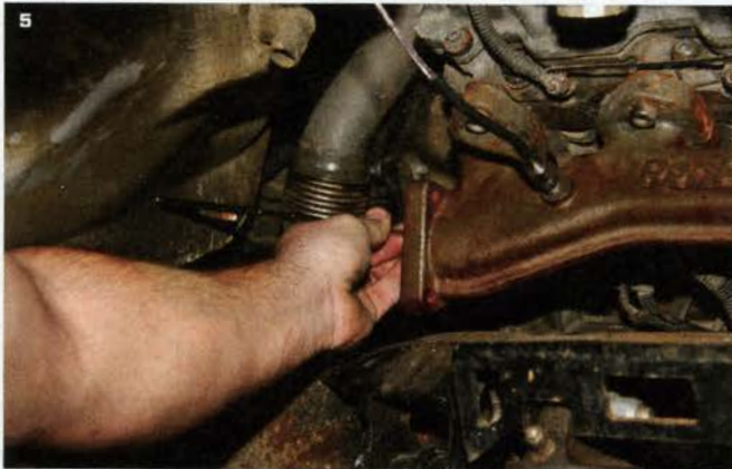
5 Then, to make sure that no metal particles get blown into the new turbo, he removes the up pipe and uses a magnet to clean out any metal shavings from the manifold.
