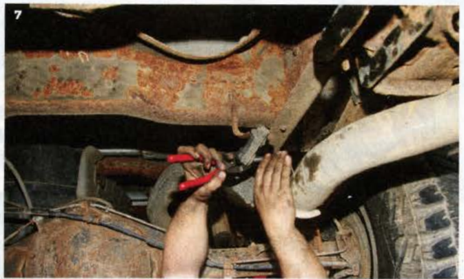
7 To remove the rear section of the exhaust system, Bruner uses a large set of pliers to pop the hangers out of the rubber grommets. He then works the old pipes out from under the truck. On a truck with less ground clearance, you may need to cut the old system to make it easier to get it out from under the truck.
