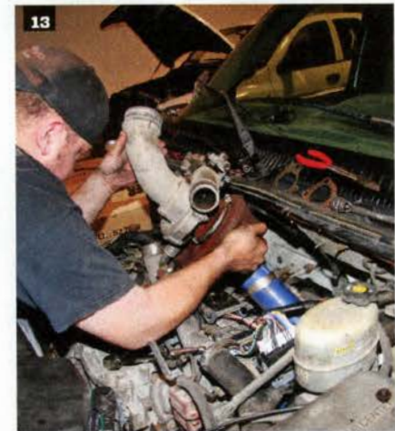
13 After removing the factory downpipe and unbolting the up pipes, Newton unbolts the turbo and its water and oil lines and then removes the turbo from the Duramax.
