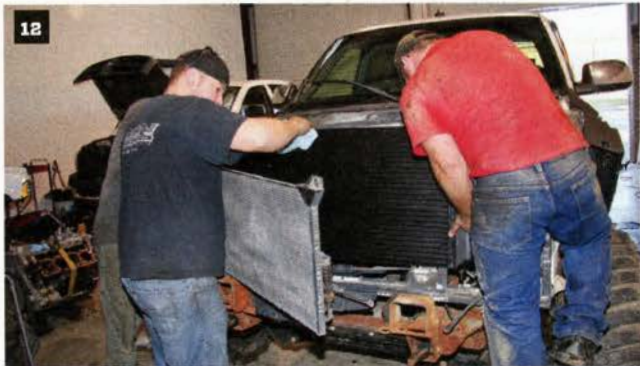
12 The new larger Banks Power Techni-Cooler is installed next.
