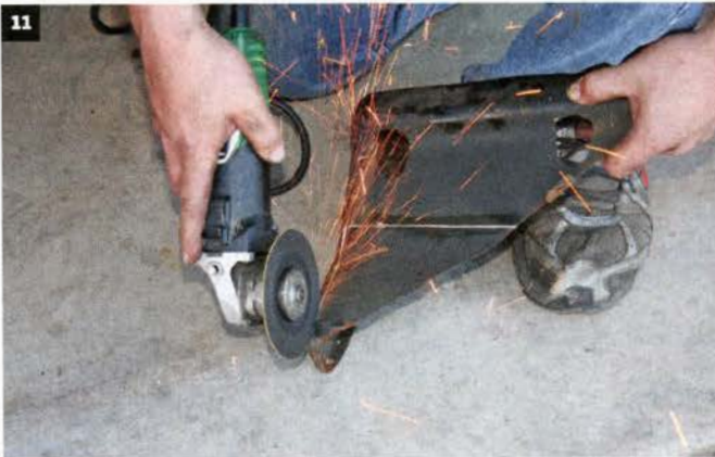
11 After marking the airbox support bracket with the supplied template, Newton trims away the lower part of the bracket to make room for the larger boost tube.
