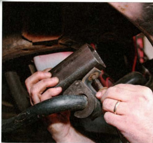
To allow the new intercooler to fit, Banks supplies you with two blocks to lower the sway bar the 2 inches it needs to fit properly.
