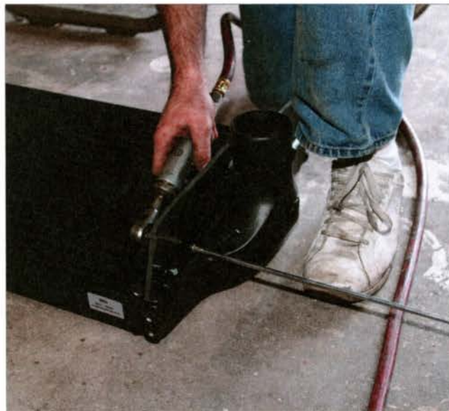
Here, we installed the heat shields. This will help prevent engine heat from reaching the intercooler.
