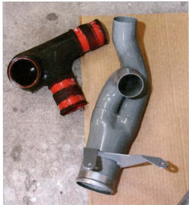
Once the stock "Y" pipe was removed, the new one could be installed. Here is a picture of the stock version (left) and the Banks version side by side.
