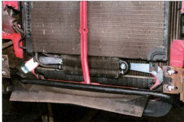
Next to be installed were the trans cooler mounts. Yes, you do have to relocate the trans cooler. Banks supplies the brackets. You may also notice the bumper was removed to allow more room to work.
