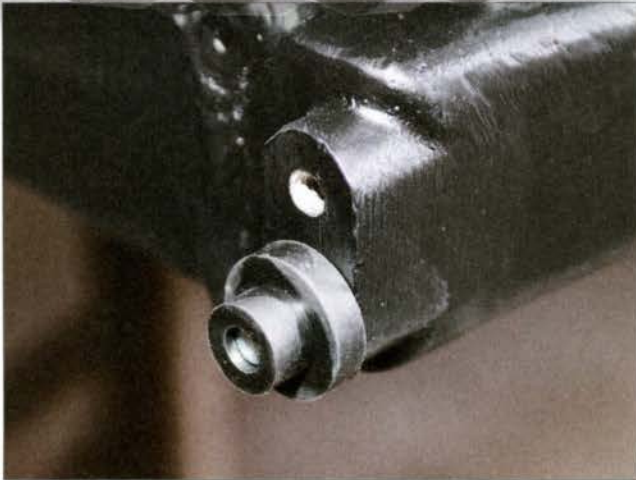
Here are the lower intercooler mounts after they were installed.
