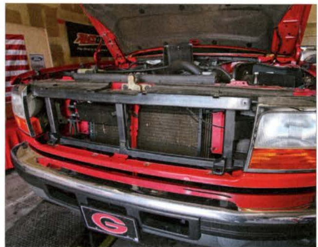
To begin the disassembly, Bill Cohron removed the front grille.
