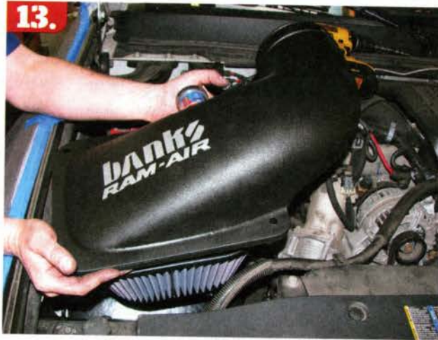
13. After mounting the reusable filter to the base of the huge lid, the assembly was set into place over the lower filter housing.
