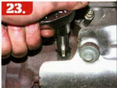
23. Monitoring Exhaust Gas Temperature (EGT) is imperative in a performance diesel application. We had to drill and tap a hole in the GMC's passenger-side exhaust manifold to allow a probe to be mounted.
