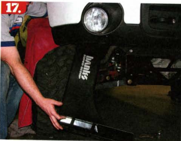
17. Our truck's large lift and tall tires made slipping the Super Scoop up the narrow passage between the inner fender and core support a breeze.
