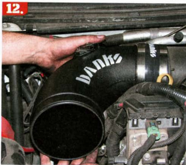
12. The mandrel-bent intake pipe and flex coupler were next. It was mounted onto the turbo's original intake tube and does not do away with the air silencer, as testing showed no need for modifications there.
