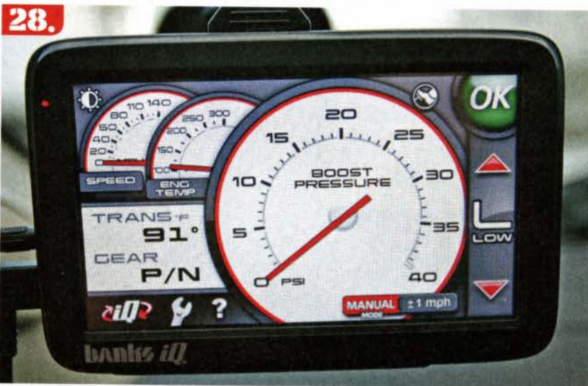
27. & 28. The brains for the Six-Gun and SpeedBrake were stuck to the truck's fuse and relay center under the hood. We made sure all the added wiring was routed in a clean manner away from anything that might damage it. Inside the cab, the IQ 2.0 Man-Machine interface was mounted to the windshield. From here, we will be able to listen to music while setting the SpeedBrake for towing, choosing a power level for blasting down the road, and monitoring the backup camera when reversing.
