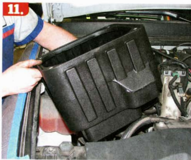
11. All that room allowed the Ram Air base to be dropped in and bolted down.
