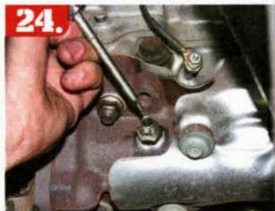
24. After threading a tubular insert into the new hole, the EGT probe was coupled to the insert. The probe's harness was then added to the Six-Gun tuner.
