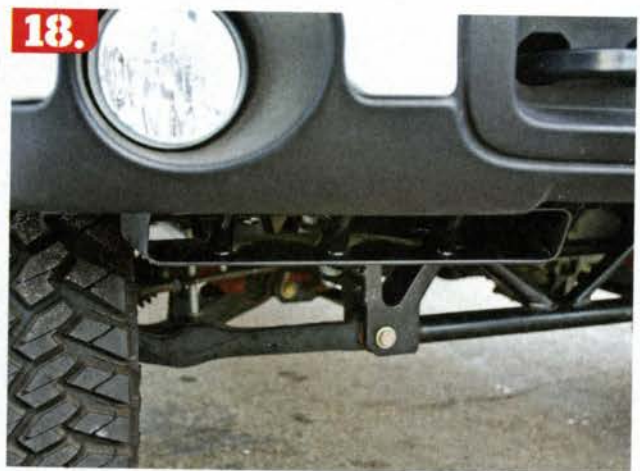
18. In final position and bolted on tightly, the Super Scoop is barely noticeable yet delivers a plentiful supply of oxygen-rich, dense air up into the Ram Air box.
