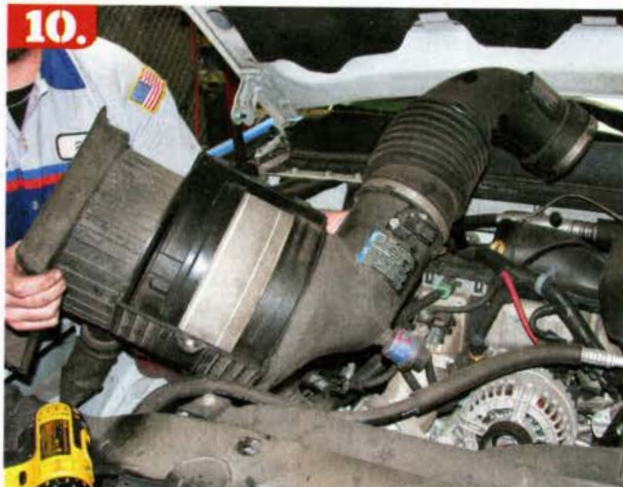
10. After popping the original air intake from the truck, it was apparent that it was in need of some attention. Be sure to check your filter more often than we did.
