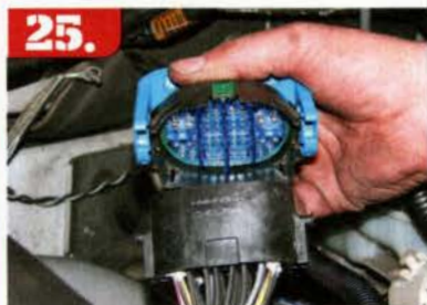
25. To gather all the Duramax's information, the Six-Gun tuner simply plugs in inline with the original ECM cabling and MAP sensor. The SpeedBrake harness was routed down to the transmission harness underneath the truck.
