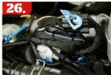
26. As you can tell, the Six-Gun harness is quite extensive, pulling information from all the factory senders including the, IAT, MAF, TPS, coolant temperature, oil pressure, fuel level, transmission temperature, and many more. All this is required to create plenty of power in a safe manner.
