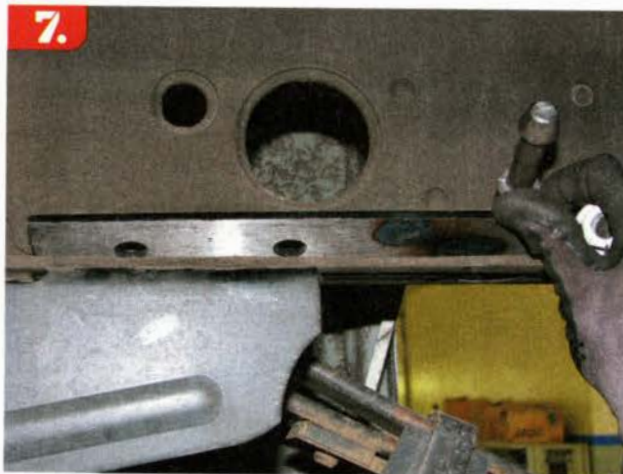
7. Since the driver side does not normally have an exhaust outlet, Banks designed this ingenious hanger to support the tubing. It bolted into the frame with the stock hardware holding the trailer hitch into position.
