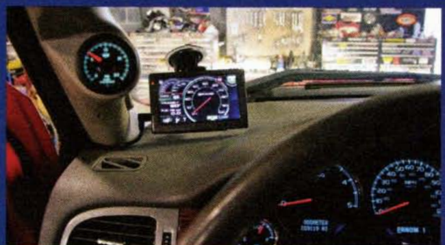
The 5-inch touch screen is easy to read and use. It can be configured to match your truck's gauges while displaying up to five parameters.
