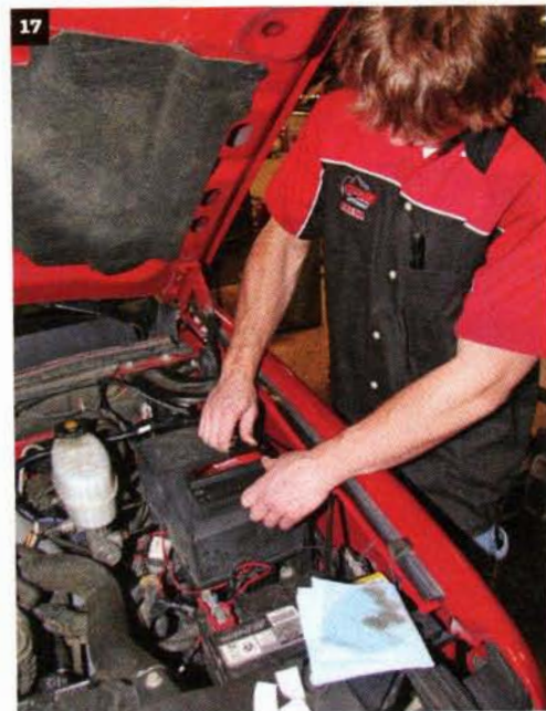
Then, he plugs the harness into the SpeedBrake module.
