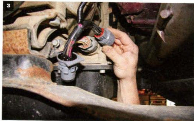
3 To keep the harness out of harm's way, he passes it over the top of the transmission housing to get it to the connector on the rear passenger's side of the transmission housing. The harness from Banks Power uses connectors that plug directly into the factory connectors for an easy installation and without slicing up the factory harness.
