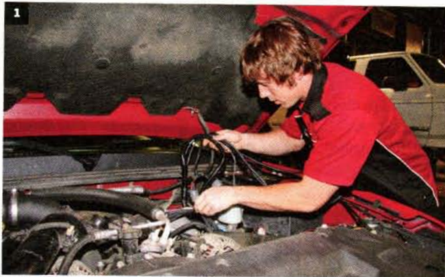
1 Michael Powell starts the installation by laying out the new wiring harness under the hood in the general area it will be installed. Then, he runs the transmission intercepting harness down to the transmission, following the factory harness routing.
