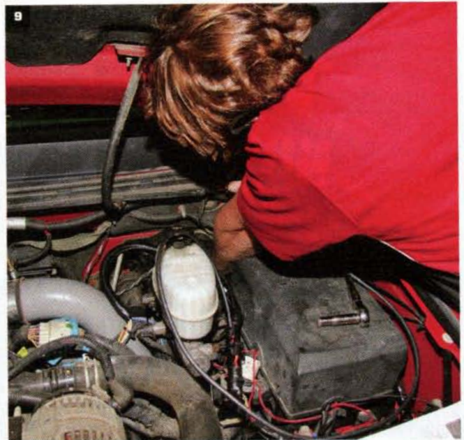
Powell passes the end of the harness into the cab of the truck through a small slit in the factory rubber grommet. Be careful not to cut any wires when cutting the slit in the grommet.
