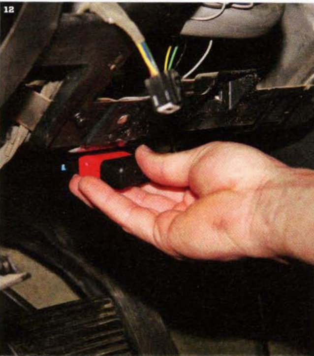
The OBD-II interface connector plugs directly into the OBD-II port under the dash.
