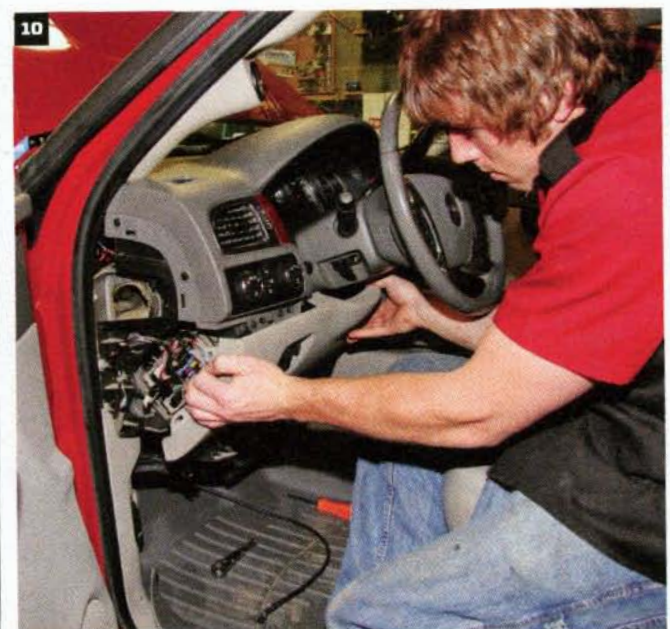
Moving into the cab, Powell removes the fuse panel access cover, as well as the lower dash panel.
