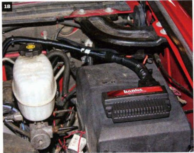
To finish off the installation, Powell secures the harness to the factory harness using zip ties for a clean and safe installation.
