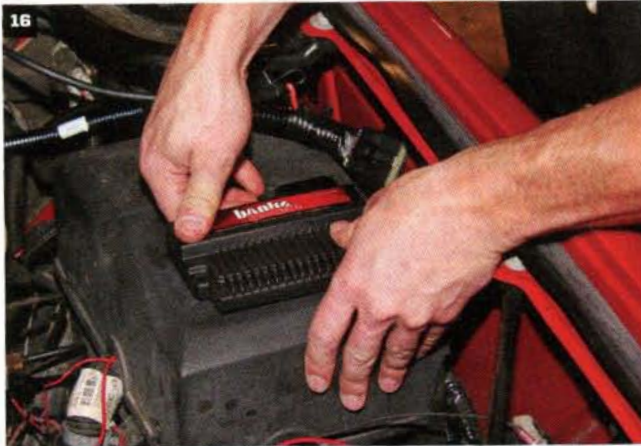
After cleaning the top of the fuse box cover under the hood, Powell mounts the SpeedBrake module using the supplied hook-and-loop strips.
