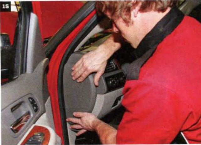
Now, he reinstalls the lower dash panel and fuse panel to complete the interior part of the installation.
