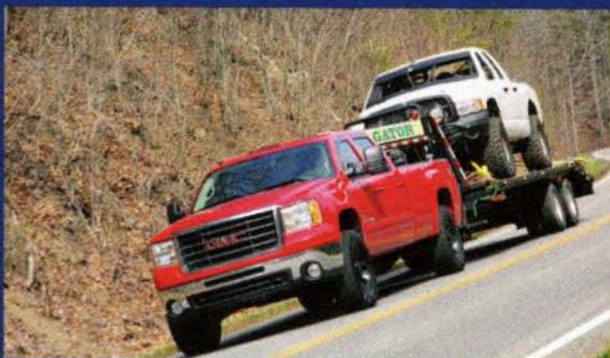
The GMC 2500 HD has big brakes, but with the SpeedBrake activated, you can keep them cool and ready for action while letting the engine and transmission provide the braking.
