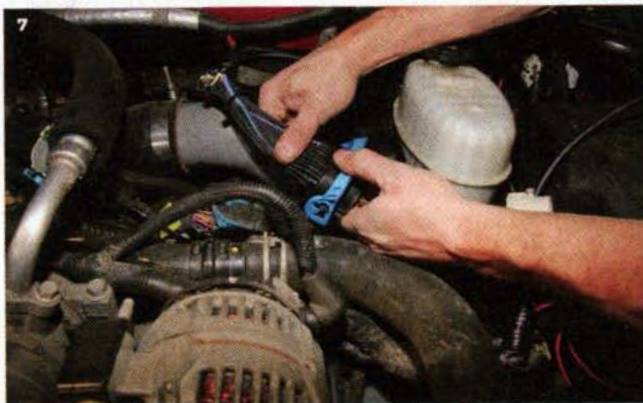
6 & 7. Unplug the black connector and install the Banks Power intercept harness between the two ends of the black harness connectors. Don't forget to reconnect the white connectors before moving on to the next step.
