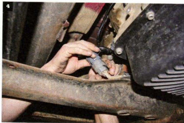
4 Simply unplug the transmission connector and plug the Banks harness connector into the transmission. Then plug the transmission connector into the Banks harness. Be sure to secure the harness with the supplied zip ties to keep it away from hot and moving parts.
