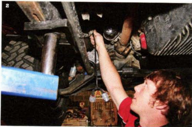
2 Using a hoist, Powell lifts the truck into the air to run the transmission portion of the harness, but you could do this on the floor of your garage.
