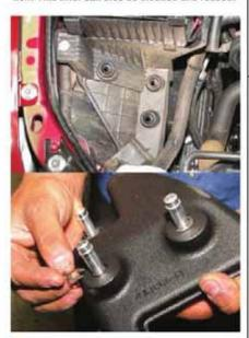
2. The entire stock air intake system is removed and is replaced by the Ram-Air system. Here's the inner fender mounting location. Banks has designed their air filter box to be a simple push in like the original. These three aluminum pins are held in by C-clips and are the secret to this like stock ease of installation system.
