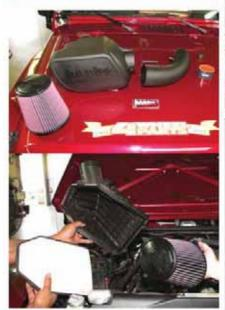
1. The Banks Ram-Air features a closed top air box. This design keeps the filter cleaner and also improves air flow velocity to the filter and on through to the engine. The stock flat-panel air filter is replaced with a Banks conical filter that offers more surface area and better filtration. This filter can also be cleaned and reused.
