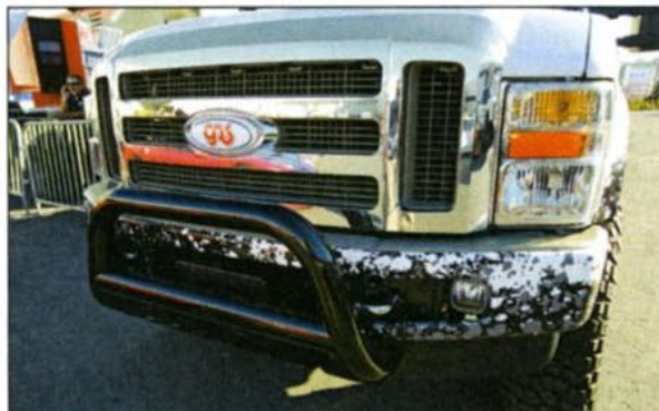
Since the new Ford trucks house seven radiators up front to cool various engine fluids, a Smittybilt Grille Saver was installed to protect them from off-road obstacles.
