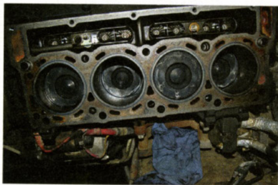
1. This is what the left side of our 6.0 looked like after the heads and gaskets were removed.
