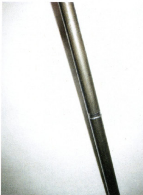
13. The pushrods were all the right length and showed very little wear, with the exception of this one, which was badly galled and had to be replaced.
