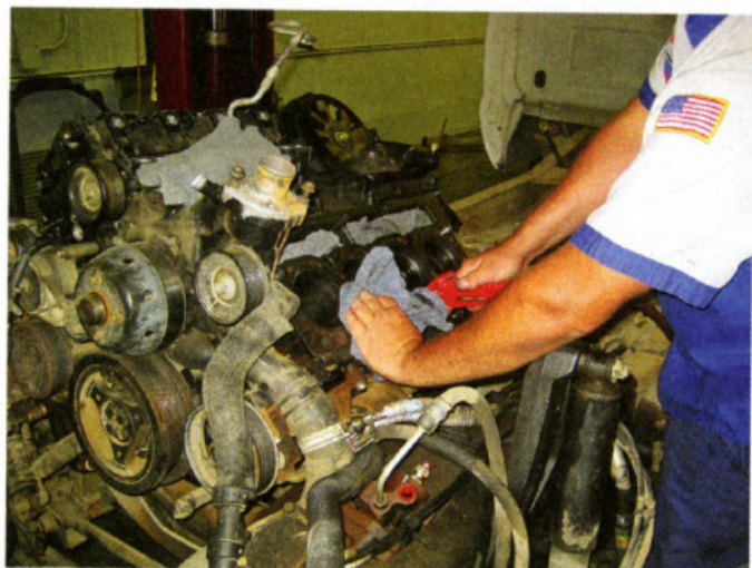
3. With the lifters covered, the threads for the new head studs were blown out to make sure there was no fluid inside that would prevent perfect thread engagement.
