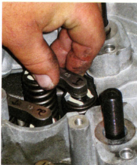
15. Next, the valve bridges are installed. They were marked with indelible pen when they were disassembled, so they can be reinstalled in exactly the same position.
