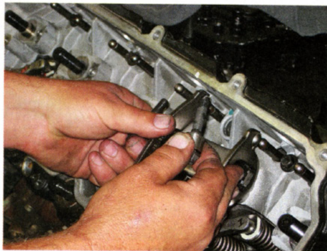
16. After rotating the crankshaft by the harmonic dampener so the locating notch is in the 6 o'clock position, the rocker arm assemblies can be installed.
