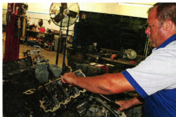
24. After the inner cylinder head studs are torqued in sequence, the outer bolts are torqued in two stages. With this process and use of new parts, our 6.0 should keep its gasket in place. From here, what remains is to install the glow plugs, the fuel injectors, the intake manifold, EGR cooler and the turbo ... which we'll show you next month.
