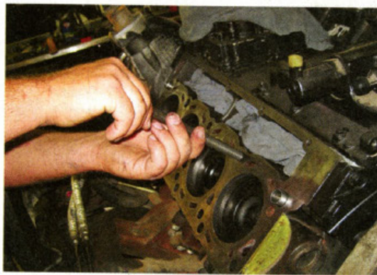
4. Just to be sure, our mechanic carefully chases the threads so that the studs will be installed with maximum thread contact.
