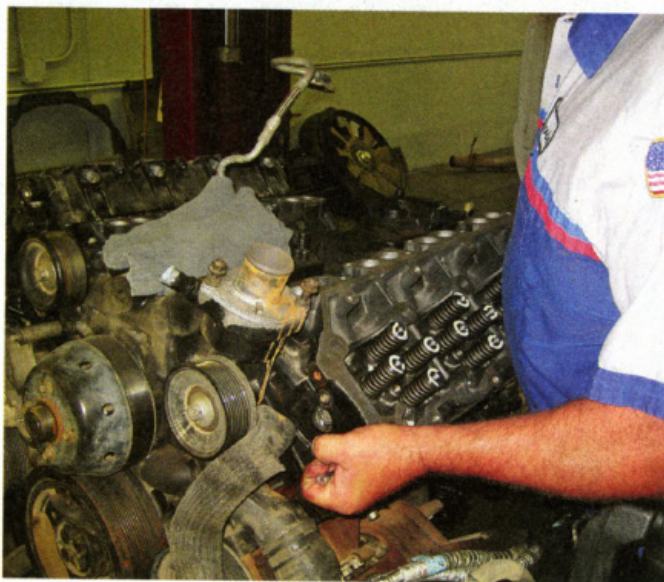
6. Our mechanic installs the cast-iron cylinder head using screws installed at the ends of the rebuilt head as helpers. Then he removes the lifting screws.
