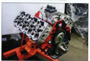
The additional bore of the engine allowed Fleece to utilize large, 35mm intake and exhaust valves, which will be essential in allowing the big-cubic-inch Duramax to breathe properly. SoCal Diesel provided the stainless steel intake valves, Inconel exhaust valves, springs, retainers, and 0.083-inch-wall-thickness chromoly pushrods.
