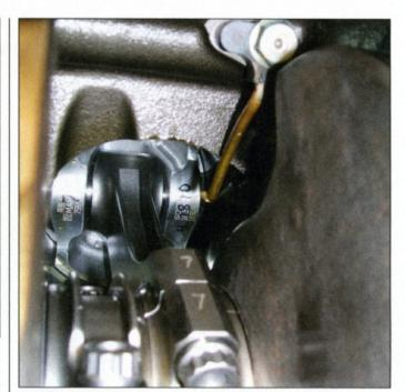
Forged Carrillo connecting rods and forged pistons from Mahle round out the rotating assembly. The pistons feature custom fuel bowls designed to excel with a short-duration combustion process. The pistons were also fly-cut to match the increased-duration camshaft. In addition, Fleece reworked the factory piston cooling oil jets (boring them larger) for increased oil flow to the bottom of each piston.
