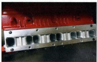
The stock, aluminum cylinder heads were CNC-ported and received a three-angle valve grind, and fire-rings were cut and installed (fire-ring grooves were also cut in the block). Cylinder head cooling will be handled by a Meziere Enterprises electric water pump. Glow-plug-deleting plugs from SoCal Diesel were also threaded into each cylinder head.
