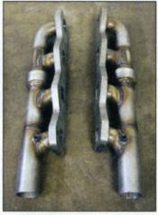
A set of ProFab Performance headers built by Rick Lance will direct exhaust from the cylinder heads toward the front of the engine, in order to work with the custom turbocharger system (where the compressor will face the firewall for the shortest intake path). All exhaust plumbing will be ceramic-coated before being installed in the vehicle.
