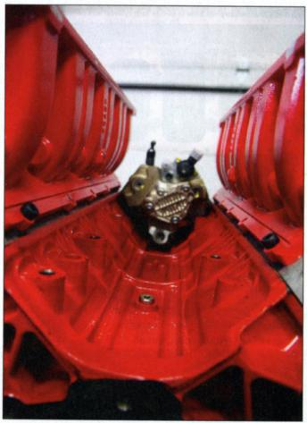
Twin 150-gph AirDog fuel systems will supply fuel to two CP3 injection pumps. Both CP3s are Industrial Injection units that are rated to flow 120 percent more than stock. The first CP3 will retain its factory mounting location (at the front of the lifter valley), while the second pump will be driven via a custom accessory beltdrive.
