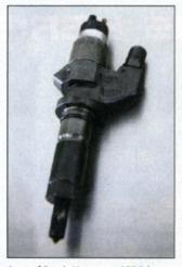
A set of Bosch Motorsport LBZ injectors flowing 385 percent more fuel than the factory units will deliver diesel into each cylinder. Short duration is the strategy here—lots of fuel will be delivered very fast. According to Fleece, these injectors are designed to maximize fuel delivery for short-duration, high-rpm applications.
