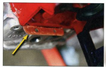
In this high-performance application, solid copper head gaskets were used for the best seal possible between the cylinder heads and the block (arrow), and also because factory gaskets aren't available for the bore size of each cylinder in this particular application. A set of ARP 625 head studs secure the heads to the block.
