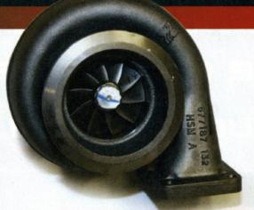
A huge, 10-blade, 96mm turbine (inducer dimension) wheel will sit in the big 1.32 A/R exhaust housing—that's just under 3.8 inches. The turbocharger inlet on the turbine side will be mountd via a T-6 mounting flange and spent exhaust gases will exit the turbine through a 5-inch-diameter
