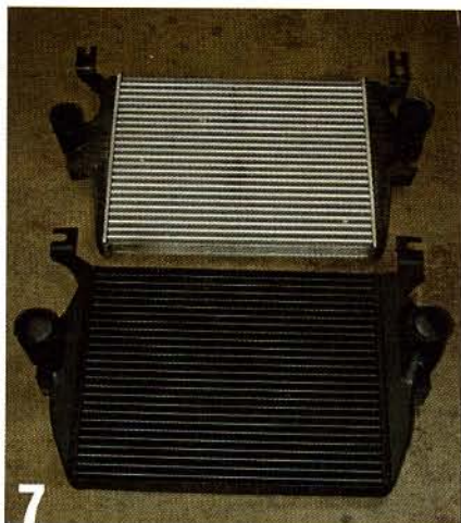
7 The intercooler's primary job is to cool the charged air prior to entering the combustion chamber. The result is more oxygenated air, which allows for more fuel to be transformed into power. A byproduct of this
