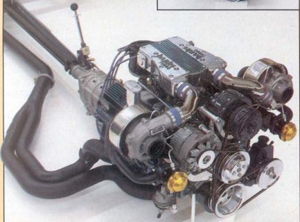
minimize noise and wear, the electric pumps only operate above 2 psi of boost. The carburetor feeds the pressurized mixture to a modified Edelbrock Torker intake manifold chosen for its conservative port design. The resulting blowthrough configuration minimizes engine height and the length of the air-fuel mixture's path to the combustion chamber.
