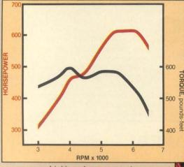
we start thinking about generating more speed. We need taller gearing, because at 6600 rpm, the engine is 75 hp below its peak output. A two-part solution materializes. We will replace the Ford rear axle with a twelve-bolt Chevrolet unit that can accommodate a 2.29:1 gearset. Then we will mount a set of Hoosier street-legal roadracing tires, which are from 1.5 to 3.0 inches taller than the Goodyears. With these changes, 200 mph should fall much closer to the engine's power peak.
