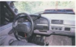
▲ The interior of Jason's Ford looks deceptively stock until you recognize that the seats came from a Dodge, that a triple-pod of gauges lives on the A-pillar, and that hidden inside are 10 stereo speakers fed by a ground-shaking audio system.
