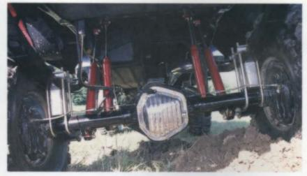
▲ Jason didn't stop at installing two Skyjacker shocks at each of his Ford's corners. He also didn't stop at painting those shocks Ford's electric Red. He also had to add extended shock mounts, which were coated with Powershield metallic coating.
