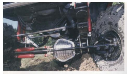
◀If that looks like a Dana 60 doing duty under the front of Jason's Ford, that's hecause it is. Jason also treated his truck to a drop pitman arm, ORU crossover steering, and dual Skyjacker steering stabilizers.
