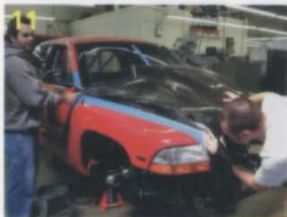
11 DESPITE NEEDING A FEW AERODYNAMIC TRICKS TO CHEAT THE WIND TO REACH 200 MPH, THE SIDEWINDER RETAINED MUCH OF THE DAKOTA'S ORIGINAL SHEETMETAL. ONE AREA THAT DID RECEIVE MAJOR MODIFICATIONS WAS THE HOOD, AS A BULGE WAS NEEDED TO CLEAR THE CUMMINS' TALL CYLINDER HEAD. HERE, A RAW FIBER-GLASS HOOD, RIGHT OUT OF THE MOLD, IS TEST-FIT ON THE DODGE.
