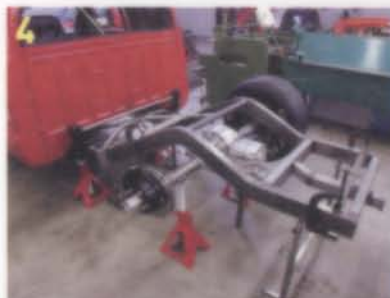
TACKETT FABRICATED NEW FRAMERAILS FROM THE CAB BACK TO CLEAR THE FAT REAR MEATS THAT THE TRUCK WOULD USE AT BONNEVILLE, AND ALSO TO HANG THE FOUR-LINK REAR SUSPENSION. IN THIS PHOTO THE QUALITY MACHINE QUICK-CHANGE REAREND IS IN PLACE, THOUGH THE FOUR-LINK WOULD ALSO HOOK UP TO A TRACK 9 GRAND NATIONAL 9-INCH REAREND. NOTE THE RECEIVER HITCH CHANNEL BUILT INTO THE FRAME. BANKS PLANNED ON SIDEWINDER TOWING ITS OWN PARTS TRAILER ONTO THE SALT.
