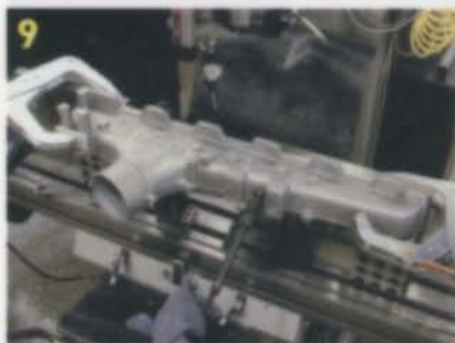
9 BECAUSE OF THE SPECIALIZED NATURE OF THE CUMMINS, MANY OF THE COMPONENTS NEEDED TO BUILD THE MOTOR HAD TO BE FABRICATED OR HEAVILY MODIFIED AT BANKS' FACILITY. HERE, A RAW BANKS BIG HOSS INTAKE MANIFOLD CASTING UNDERGOES MACHINING.
