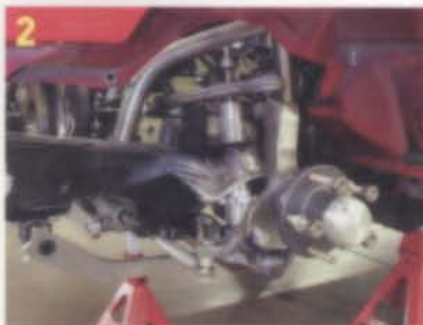
THERE WASN'T AN AFTERMARKET SUSPENSION KIT APPROPRIATE FOR THE DAKOTA'S PERFORMANCE ENVELOPE, SO SIDEWINDER PROJECT LEADER SHELDON TACKETT BUILT ONE. THE FRONT SUSPENSION UTILIZED FABRICATED TUBULAR-STEEL CONTROL ARMS, MODIFIED BUSCH GRAND NATIONAL SPINDLES AND HUBS, AND HEIGHT-ADJUSTABLE PROGRESS GROUP COIL-OVERS. HERE YOU CAN ALSO SEE THE BRACKET FOR THE TORSION-BAR-TYPE FRONT SWAY BAR FROM SPEEDWAY ENGINEERING. TACKETT SET IT UP THIS WAY SO HE COULD INTERCHANGE FROM LIGHT TO HEAVY BARS DEPENDING ON WHAT SORT OF COMPETITION THE SIDEWINDER WOULD BE RUNNING IN.
