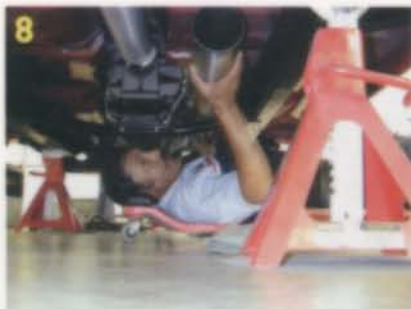
8 HERE'S ANOTHER VIEW OF THE TUNNEL-LIKE, 4-INCH EXHAUST PIPE LEADING FROM THE ENGINE.
