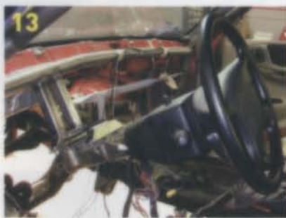
13 THERE ARE TWO THINGS OF NOTE HERE. ONE IS THE CROSS-BRACE STRETCHING ACROSS THE COWL. THAT'S PART OF THE SAFETY CAGE TACKETT BUILT FOR THE DAKOTA. THE OTHER IS THE SUPPORT BRACKET FOR THE STEERING COLUMN, NECESSARY BECAUSE OF THE STEERING WHEEL SETBACK. THE FIREWALL WAS HACKED AWAY AND THE INSTRUMENT PANEL MOVED BACK SOME 14 INCHES TO MAKE ROOM FOR THE TURBODIESEL.
