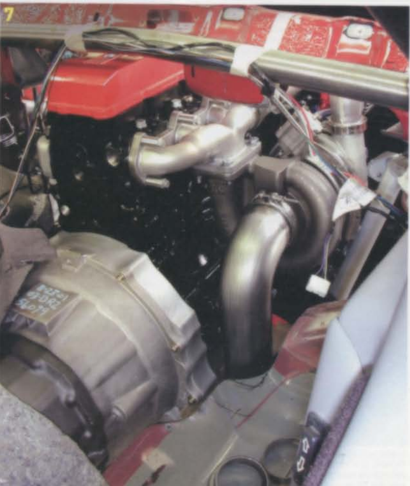
THERE'S A LOT TO SEE IN THIS PHOTO, INCLUDING THE MASSIVE HOLSET HY55 VARIABLE-GEOMETRY TURBOCHARGER, THE SEWER-PIPE-SIZE DOWNPIPE LEADING FROM IT, AND THE FRONT OF THE PROTOTYPE NV5600 SIX-SPEED TRANSMISSION. ALSO NOTICE HOW FAR BACK THE ENGINE IS SITTING IN THE TRUCK. THAT RED LINE OF SHEETMETAL AT THE TOP OF THE PHOTO IS WHERE THE ORIGINAL FIREWALL WAS CUT AWAY.
