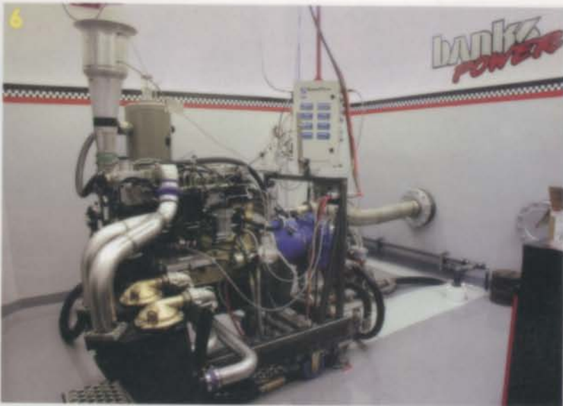
HERE'S THE BASELINE "SALT QUAKE" 5.9L CUMMINS TURBODIESEL ENGINE ON BANKS' NEW COMPRESSION IGNITION ENGINE DYNO. THE CELL WAS BUILT TO HANDLE ENGINES PUTTING OUT UP TO 1,000 HP AND 3,000 LB-FT OF TORQUE. IN THIS CONFIGURATION, THE CUMMINS WAS PRODUCING "ONLY" 393 HORSES AND 600 LB-FT OF TORQUE. BY THE TIME IT APPEARED IN RACING TRIM, THE MOTOR WENT UP TO MORE THAN 700 HP AND 1,200 LB-FT OF TORQUE.
