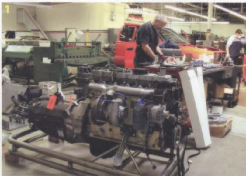
PROJECT SIDEWINDER WAS BUILT AT GALE BANKS ENGINEERING IN AZUSA, CALIFORNIA, ALONGSIDE OTHER INTERESTING GO-FAST PROJECTS SUCH AS A TWIN-TURBOCHARGED MERCEDES-BENZ DRAG RACE CAR AND A STREETABLE 200-MPH '89 CAMARO. IN THIS PHOTO YOU CAN SEE THE BASELINE "SALT QUAKE" CUMMINS TURBO DIESEL THAT MADE 393 HP AND 600 LB-FT OF TORQUE.
