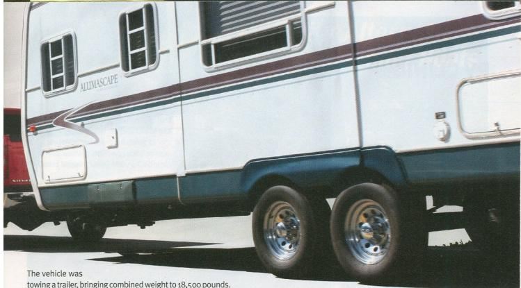
towing a trailer, bringing combined weight to 18,500 pounds. In this sequence, the tow/haul mode was activated, which also activates the Automatic Grade Braking (AGB) feature.
