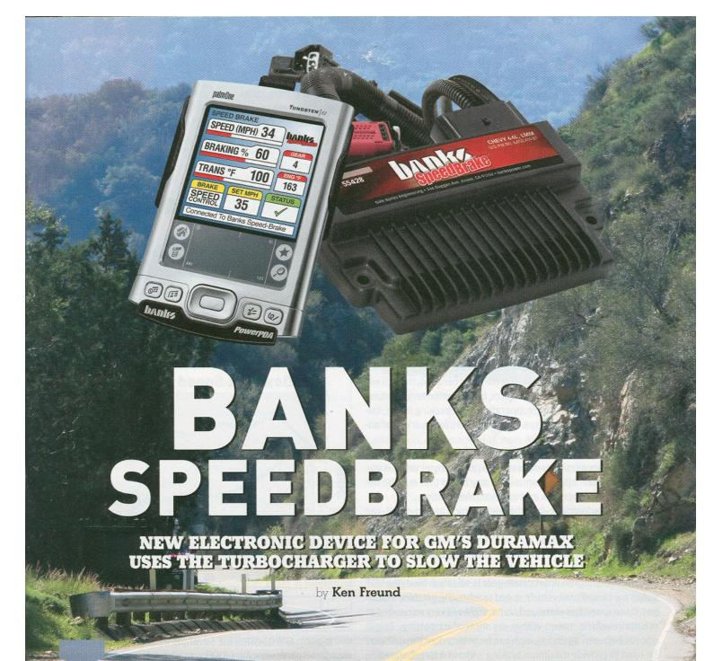
n recent years the diesel engines used in pickups have changed significantly, becoming cleaner, quieter and more powerful. Yet with all these changes, diesels still don't provide much engine braking to help slow the vehicle. Unlike gasoline engines, diesels lack a throttle valve, so when the vehicle is decelerating there is little resistance to the load pushing against the engine's internal resistance to turning.
