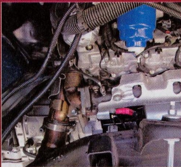
A thermocouple was installed into the exhaust manifold.
