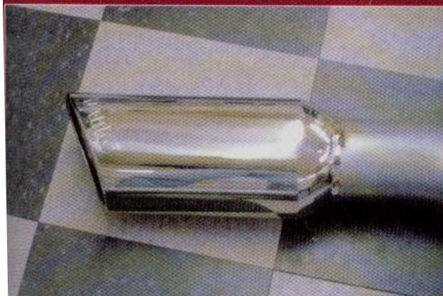
The Banks tip is a 5-inch polished stainless steel beauty with a rolled edge.
