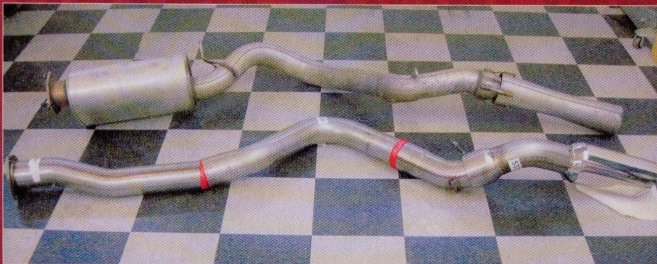
Here's a side-by-side comparison of the OEM exhaust system and the Banks Monster exhaust (foreground). The 4-inch, DPF-back system uses Cool Cuffs.
