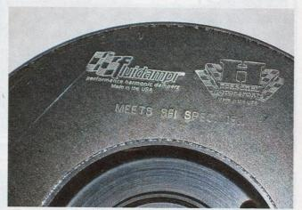
The Fluidampr, aside from never wearing out, has the advantage of being suitable for racing. The SFI spec 18.1 is stamped on the side.
