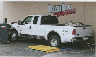
It's hard to get good rear-wheel numbers at very low RPM on automatic transmissionequipped vehicles. The transmission will downshift, rather than pull out of a full-throttle roll-on from idle. As a result, the dyno charts only show reliable data down to 2,500 RPM. Still, this truck put more power to the ground than it could have with just the Big-Hoss Bundle equipment alone — evidence that the head porting and careful reassembly was worth the effort.
