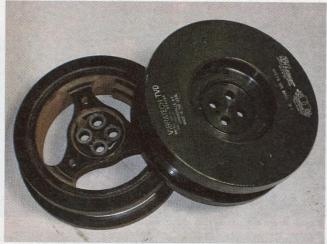
Here you can see the difference between the old harmonic balancer and the thicker Fluidampr, which is filled with silicone gel.
