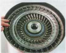
This cutaway shows the guts of the Banks Billet torque converter. The turbine and impeller assembly is furnace brazed, the turbine hub is hardened, and the pump drive is made from 4130 chrome-moly steel.
