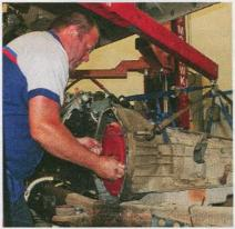
When the torque converter is fully seated, the plastic thread protectors can be removed. The bolts are torqued in three stages and require high torque values. In this case, our mechanic needed to lock up the transmission with a prybar to keep it from rotating while he tightened the bolts.
