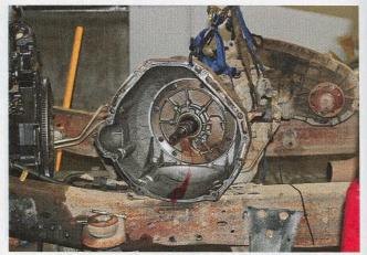
This is the transmission with the torque converter removed. To get it off, just grab it and slide it out, being careful not to let it tilt, or to damage the seal
