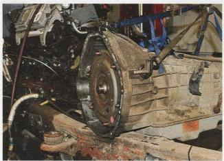
The torque converter replacement, likewise, was a whole lot easier to get at when the cab is off the chassis. Normally, the entire job would have to be done from under the vehicle.
