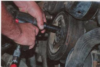
When the engine was still out of the engine compartment, Banks mechanic Kevin had an easy time pulling off the old harmonic balancer. If this replacement had been on an engine of a running truck, it would have been necessary to remove the fan and shroud as per manufacturer's instructions, and remove the accessory drive belt. Fluidampr installation instructions recommend drawing a sketch of the belt routing prior to removal if you're not completely familiar with the layout.
