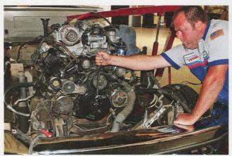
With the old unit kicked to the curb, all that remains is to properly torque the Fluidampr. The Ford bolts call for 50 lb-ft, plus a 90-degree turn. If you were working in the tighter quarters of the engine compartment, you would have to route the accessory drive belt between the Fluidampr and the water pump pulley before installing the Fluidampr and torquing down the bolts.
